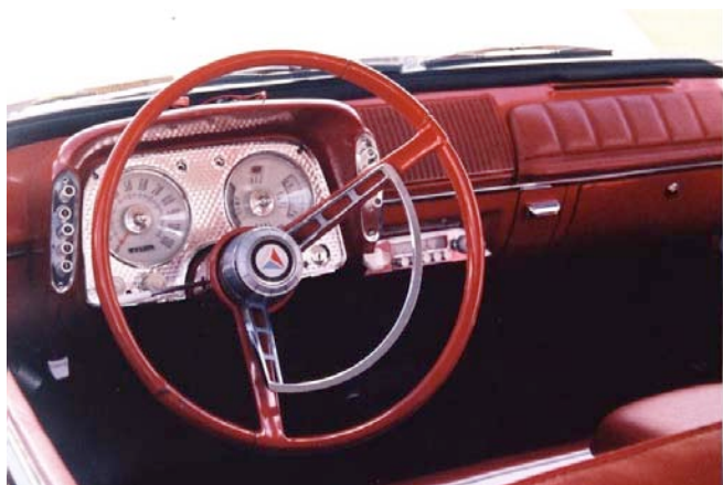
Interior of left-hand-drive Plymouth Valiant (US Version of "R" Series). Push-button automatic transmission was a feature of some cars of the era. [R. Kerr. 2005.]
